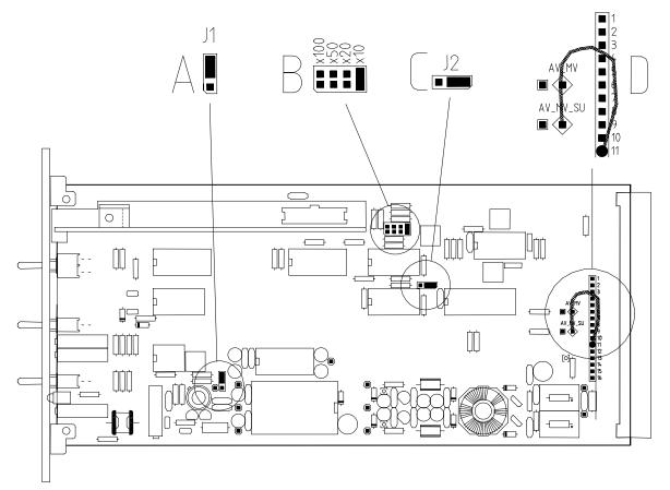
Fig. 2: Position of the internal links
