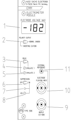
Fig.3 Controls on the front panel
